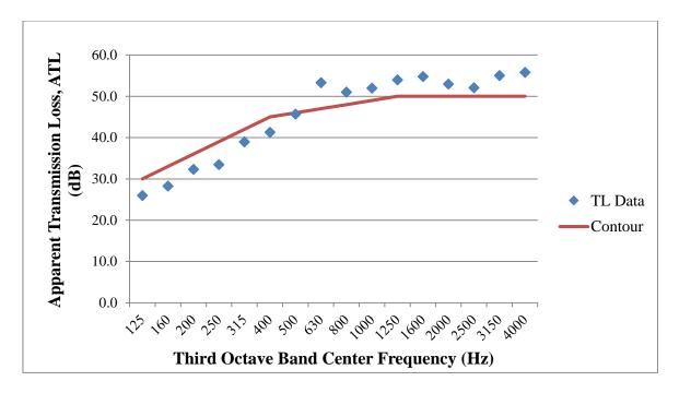
Figure 60: ATL measurement results for the partition between classrooms 120 and 121, with an ASTC of 46
