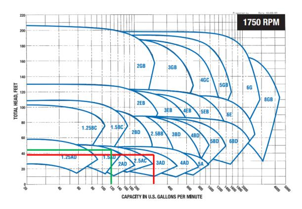
Figure 29: Pump selection diagram provided by Bell and Gossett to assist in pump sizing. Vertical geothermal pump is shown in red and horizontal geothermal loop pump is shown in green
