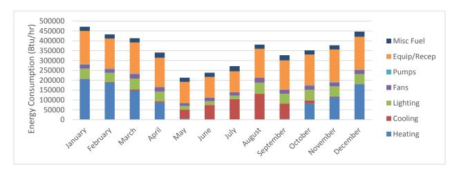
Figure 15: A graph breaking down the monthly energy consumption of the Gaige Building into the various energy consumption categories
