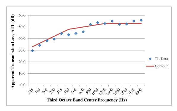
Figure 61: ATL measurement results for the partition between classrooms 121 and 122, with an ASTC of 49
