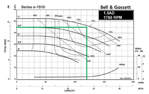
Figure 31: The pump curves shown for the horizontal loop geothermal field pump, operating conditions shown
