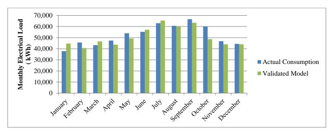
Figure 8: Comparison of actual monthly electricity consumption with results from the validated Trace 700 model
