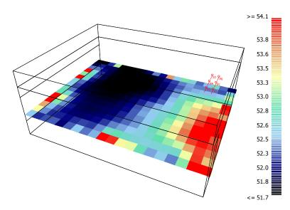
Figure 67: A grid response showing the A-weighted sound pressure levels when heat pump is running in the plenum space above the classroom
