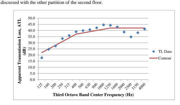
Figure 63: ATL measurement results for the partition between classrooms 247 and 248, with an ASTC of 38
