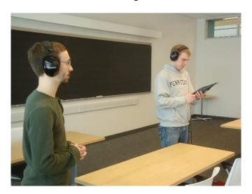
Figure 59: Sound pressure level (SPL) measurements in the 'source' room for transmission loss measurements using a B&K 2250 sound level analyzer. (AE 309 students: Aaron King and Cory Clippinger)
