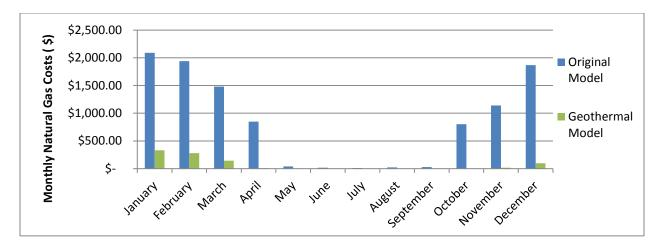
Figure 36: Monthly natural gas costs for the original and geothermal redesign of the Gaige Building
