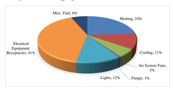
Figure 2: Annual energy distribution as calculated by the Trace 700 model used for the energy estimation of the building
