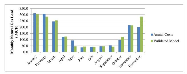
Figure 9: A comparison between the utility data for natural gas usage in the Gaige Building and the validated building model.
