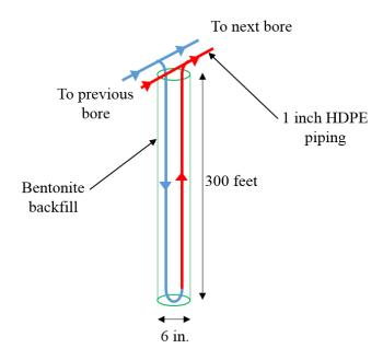
Figure 19: Specifications of a vertical well designed for the Gaige Building
