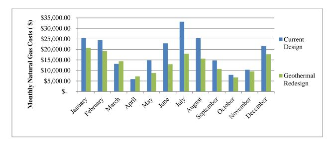
Figure 49: Annual energy cost comparison between the original campus and the geothermal redesign of the campus
