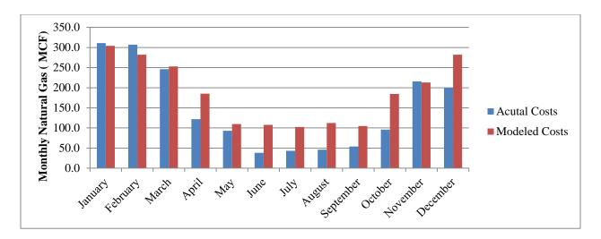
Figure 7: Actual vs. Modeled natural gas consumption on a monthly basis
