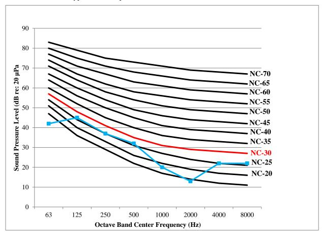
Figure 71: NC plot of background noise level from heat pump duct work for a typical office
