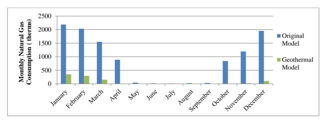
Figure 39: Monthly natural gas consumption of the Gaige Building with the original and geothermal redesign
