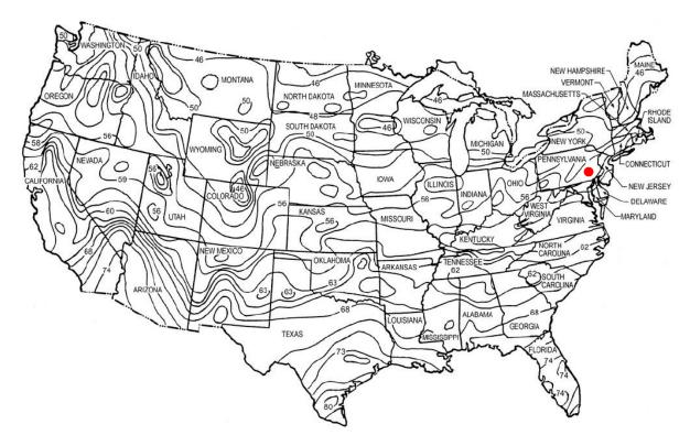
Figure 18: Undisturbed ground temperatures for the United States, Reading, PA shown at red dot
