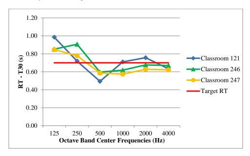
Figure 55: RT measurements of classrooms in the Gaige Building that are greater than 10,000 cubic feet
