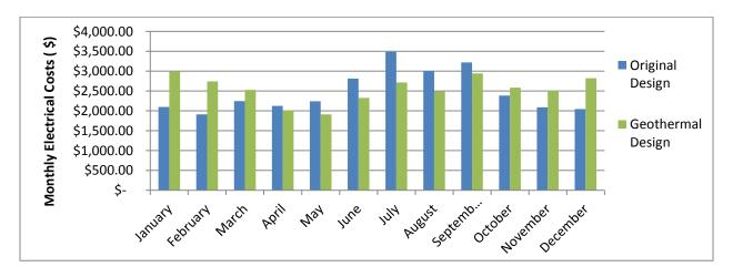
Figure 35: Monthly electricity costs for the original and geothermal redesign of the Gaige Building
