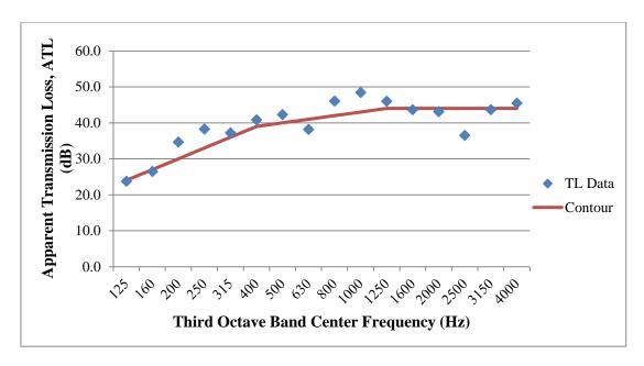
Figure 62: ATL measurement results for the partition between classrooms 246 and 247, with an ASTC of 40 The ATL measurements for the partition between classroom 246 and 247, seen in Figure 62, produced an overall ASTC of 40. This measurement is not within the level of tolerance previously described between design STC and ASTC. Details of this underperformance will be
