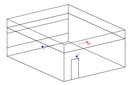
Figure 66: Source location of instructor shown in red, and receiver locations shown in blue, typical classroom
