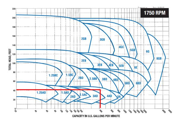
Figure 32: Pump selection diagram provided by Bell and Gossett
