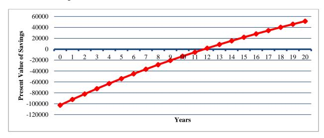
Figure 44: Life cycle cost analysis of the vertical well system for the Gaige Building
